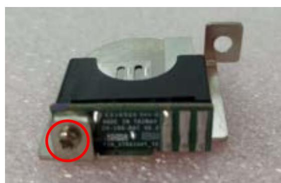
4. Pull down the indicated portion and replace the CMOS battery with a new one. (please note the battery's positive/negative pole orientation when you execute this step).
