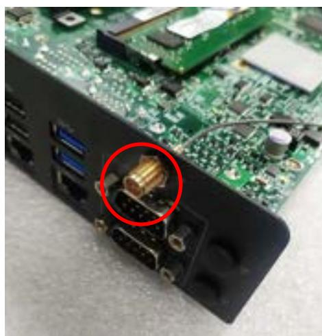
4. Assemble the antenna and antenna jack together.
