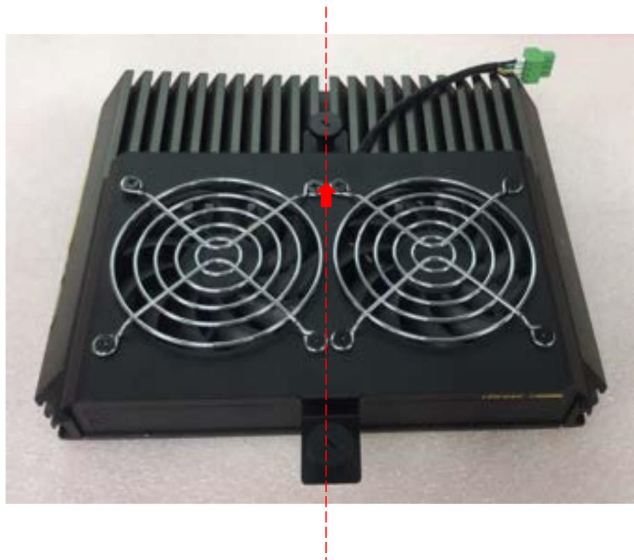
3. Move the fan to the center of chassis. Tighten the 2 screws marked on photo to secure it.
