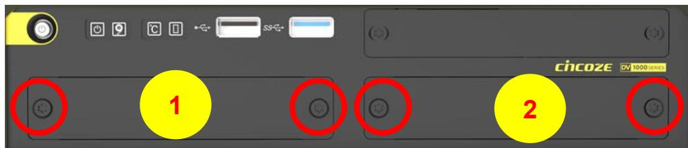
2. Attach on the MEC-USB bracket, and fasten the 2 screws to fix it as indicated.
