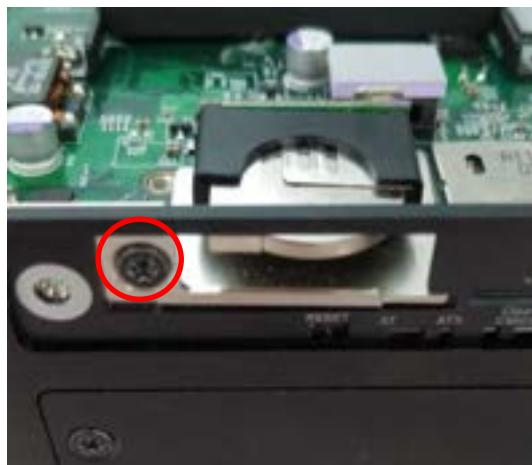
2. Pull out the CMOS battery bracket.
