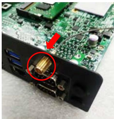
3. Put on the washer and fasten the nut of antenna jack.
