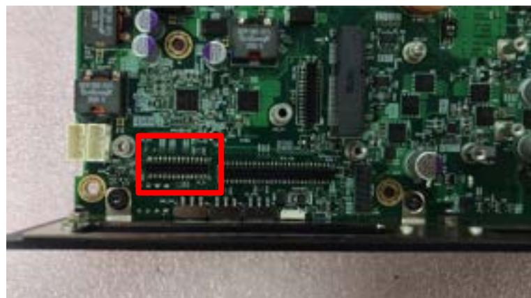
3. Fasten the two copper pillar screws as indicated.
