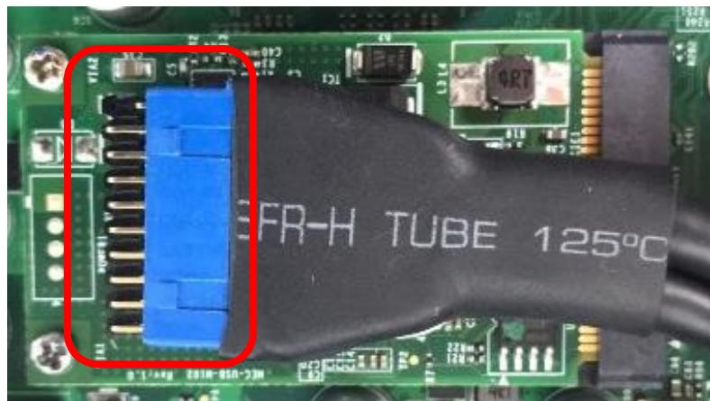
8. Attach the USB board onto the back side of the cover plate, and then fasten the two screws to secure the module.
