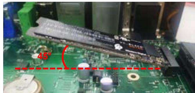
3. Press the card down and secure it with the screw.
