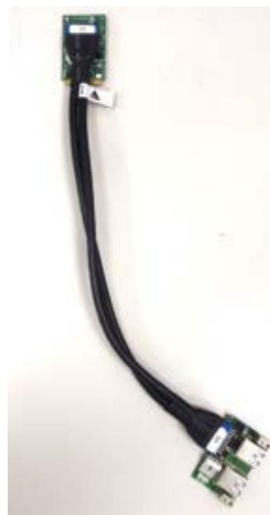
7. Connect the other end of the wire to the Mini PCIe card as indicated.
