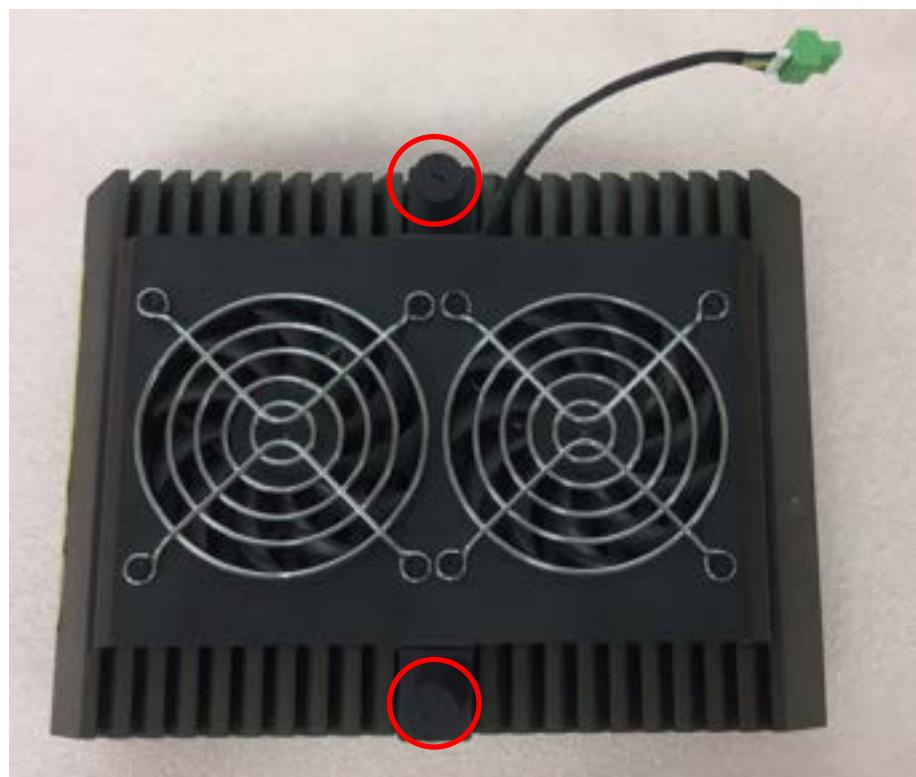
4. Connect the FAN cable to external fan power connector at rear panel.
