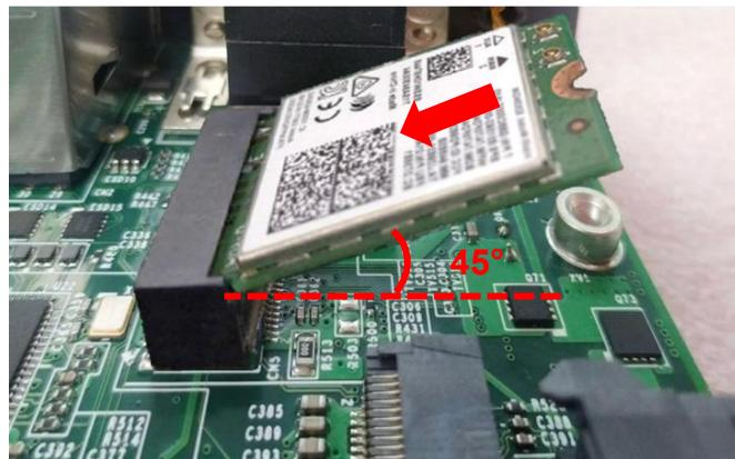
3. Press the card down and secure it with 1 screw.
