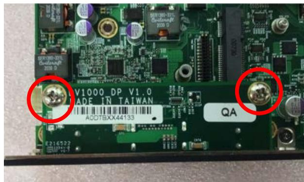
5. Attach on the CMI-DP01 bracket, and fasten the screws as indicated.
