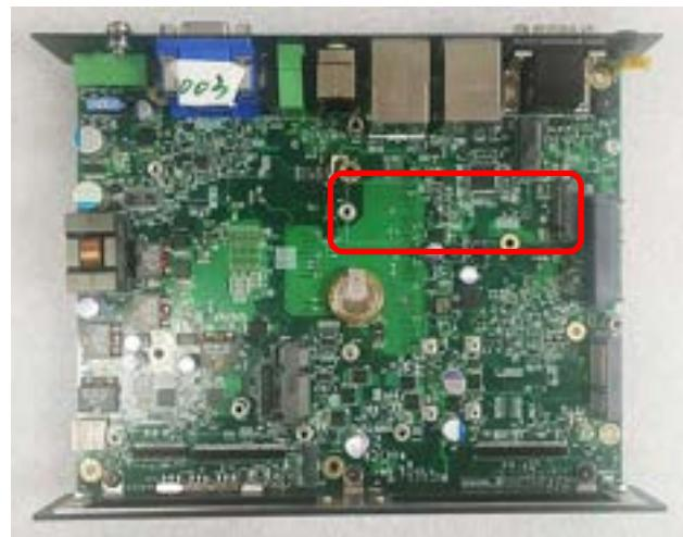
2. Tilt the M.2 M Key card at a 45-degree angle and insert it to the socket until the golden finger connector of the card seated firmly.
