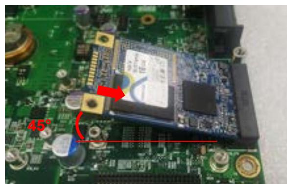
3. Press the card down and secure it with 2 screws.
