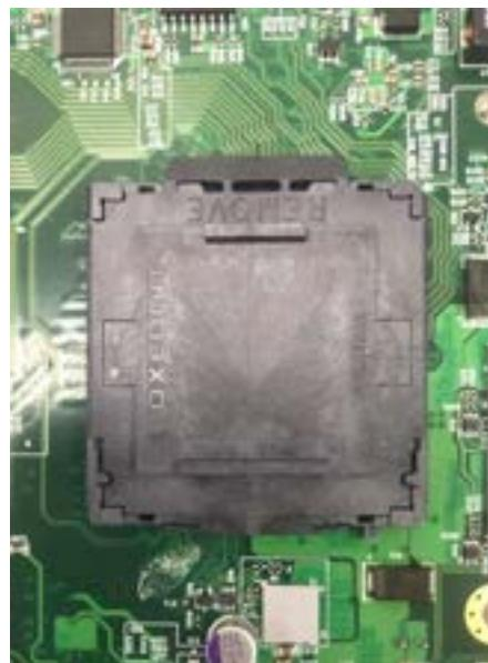
2. Insert the CPU gently by aligning the notches of the socket.
