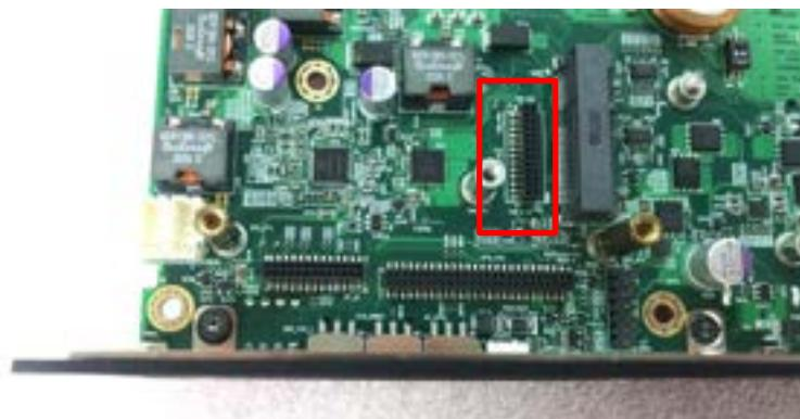
2. Insert the module vertically to the connector
