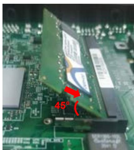
3. Press down the module until the retaining clips snap back in place.
