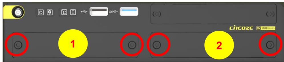
2. Attach the MEC-LAN bracket, and fasten the 2 screws to fix it as indicated.
