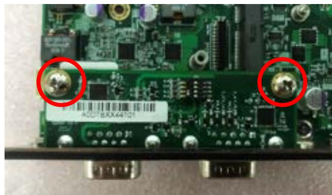
5. Attach on the CMI-COM bracket. Fasten the 2 screws and 4 D-Sub jack screws to fix it.
