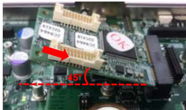
5. Press the card down and secure it with 2 screws.
