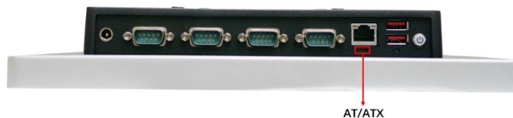
Figure 3-6: AT/ATX Switch Location
