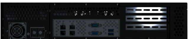
RM-2100-LB With DC Input & Full Height Expansion Slots*
