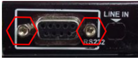
Figure 3-12: Hex Jack Screws for Securing RS-232 Connector
