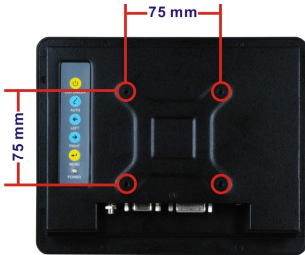
Figure 3-42: VESA Mounting Holes (DM-F65A/08A)
