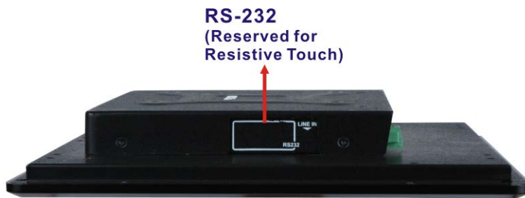
Figure 1-8: Side Panel Connector (DM-F12A/15A/17A/19A)
