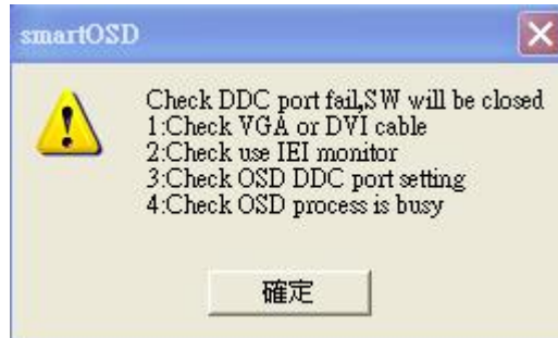
Figure C-18: DDC Port Failure
