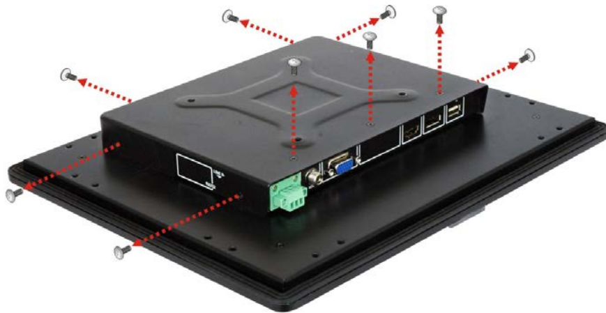
Figure 3-10: Rear Panel Retention Screw Removal (DM-F12A ~ DM-F24A)
