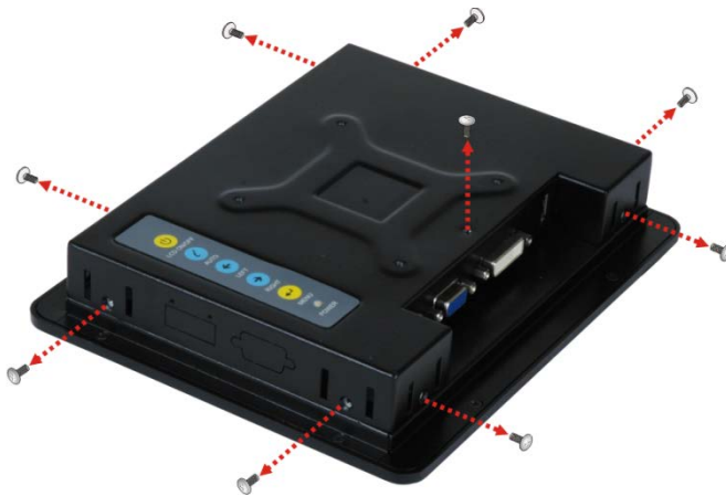
Figure 3-9: Rear Panel Retention Screw Removal (DM-F65A/08A)
