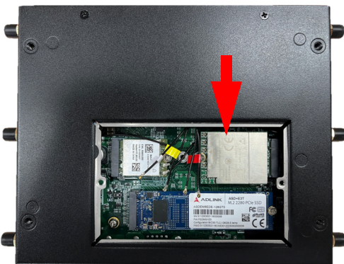
Figure 2-3: M.2 Key Slot
