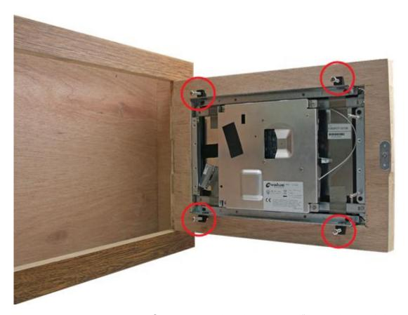
(The diagram is demonstrated by OFM-15W00, but the concept "the entire module can be secured by fastening the Panel mount screws against the wall" is the same)
