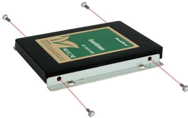
Figure 3-9: HDD Retention Screws
