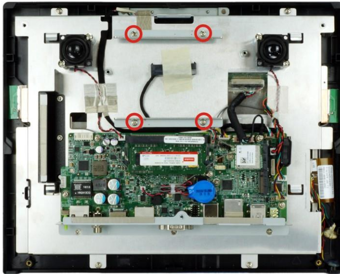
Figure 3-8: HDD Bracket Retention Screws
