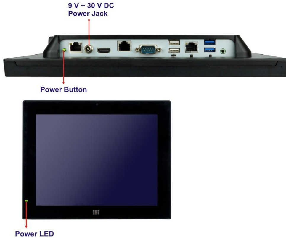
Figure 3-40: Powering On the System
