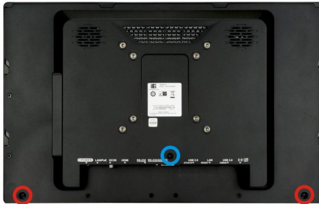
Figure 3-3: AFL3-W15A-AL Back Cover Retention Screws
