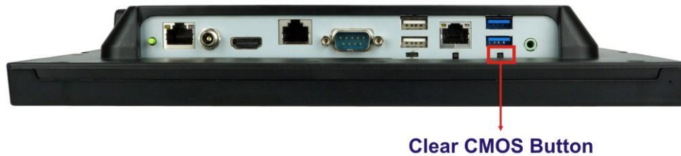
Figure 3-41: Clear CMOS Button Location
