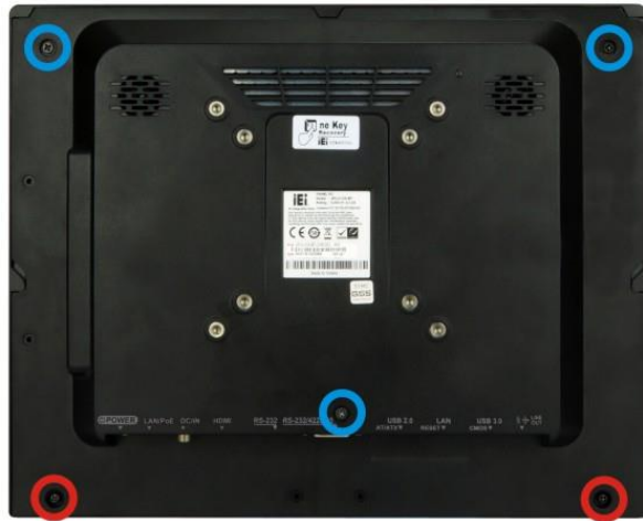
Figure 3-2: AFL3-12A-AL Back Cover Retention Screws
