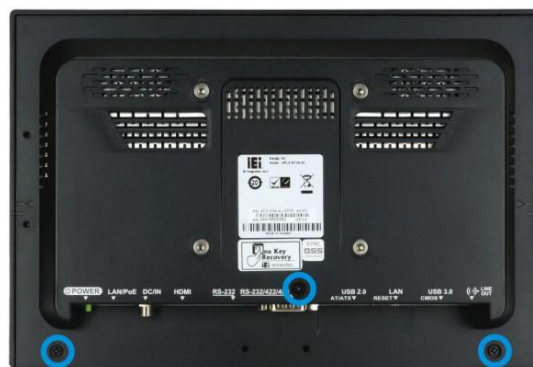
Figure 3-1: AFL3-W10A-AL Back Cover Retention Screws
