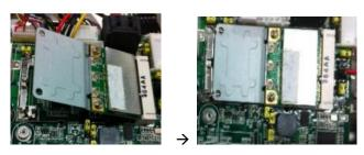
Step 3 There are two connectors on wireless LAN card. One is MAIN, and the other is auxiliary. Connect antenna cable to MAIN connector on wireless LAN card.
