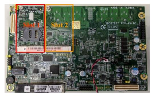
Step 2 Insert the wireless LAN card to the slot and fasten the screws as shown.
