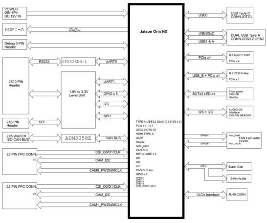
AIB-SO21/31 & AIB-SN31/41 Block diagram
