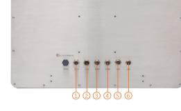
1. DC power connector 2.1 x 2.5GbE LAN 3. 1 x RS-232/422/485 (default RS-232) 8. Brightness settings +/-4.1 x RS-232/422/485 (default RS-232) 9. Power on/off 5.2 x USB 2.0
