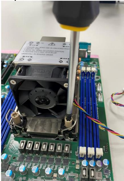
This sequence is for installing the CPU cooler above 205 Watts:
