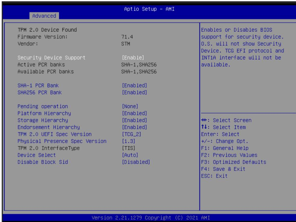
(In the Trusted Computing section, the first line will show “TPM2.0 Device Found”, if installation is successful.)
