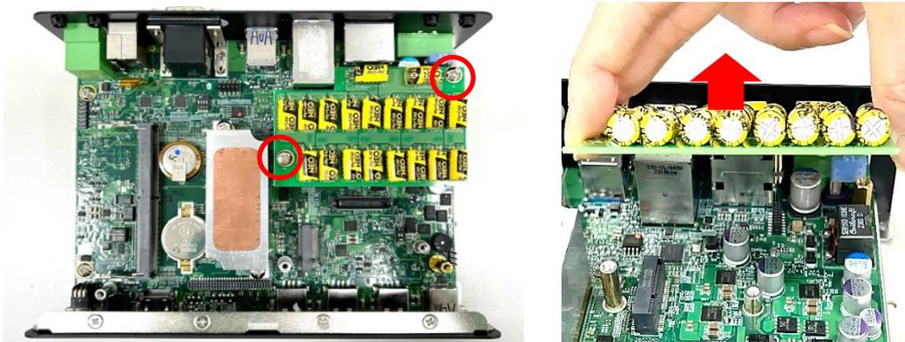
Step 2. Locate the M.2 Key E slot on the system board.
