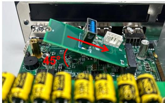
Step 3. Press down the module and fasten the screw to secure the module.
