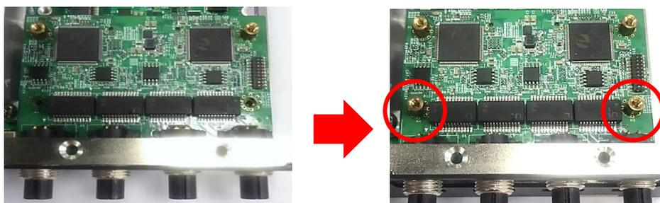
Step 3. Insert the CFM-PoE06 module vertically into the female connector on CMI module until it's connected firmly.
