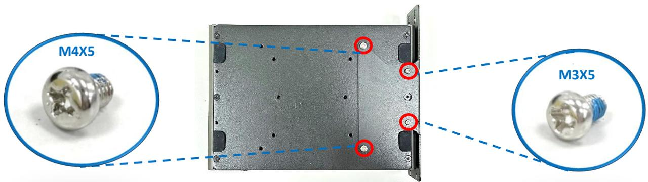
Step 2: It is feasible to secure the system to the wall by fastening the screws through the bracket mounting holes afterward.
