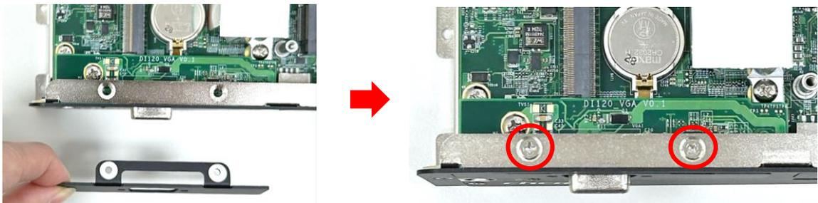
Step 6. Fasten the 2 D-Sub jack screws to fix the module. Then the installation of the module is complete.
