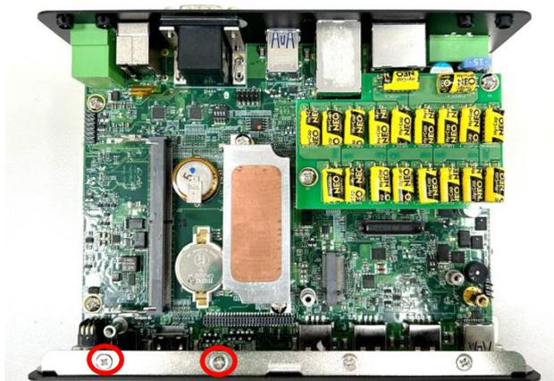
Step 3: Align the pins on the module with the connector on the right side as indicated, and then insert the CMI module vertically until it is securely connected with ensuring that the screw holes are properly aligned.
