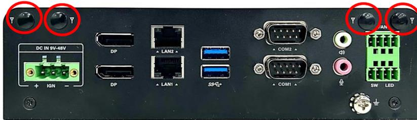
Step 2. Have the antenna jack penetrate through the hole.
