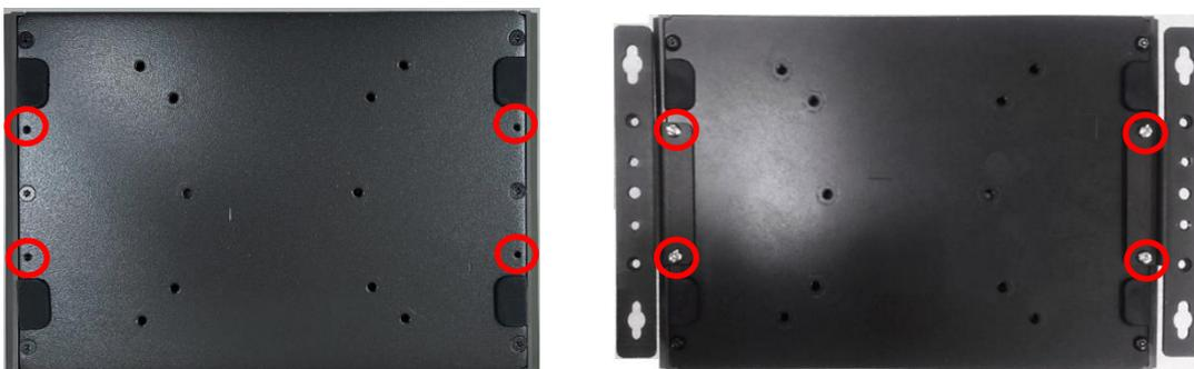
Step 2. The indicated two mounting holes at left and right sides are designed to fix the system on the wall.
