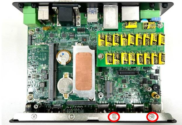
Step 4. Insert the CMI module vertically into the female connector on system's mainboard until it's connected firmly and fasten 2 screws to fix it.
