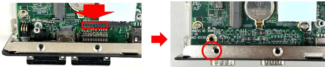
Step 4. Fasten the screw to secure it in place.
