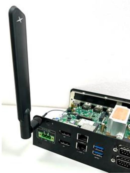
Step 5. Attach the RF connector at another end of cable onto the module.
