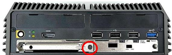
Step 3. Pull out the HDD bracket.
