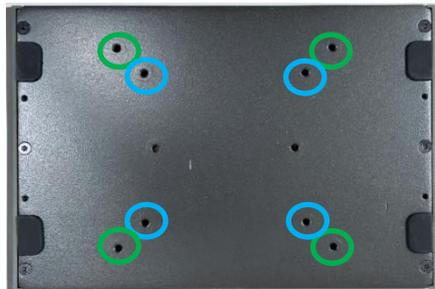
Step 1. Align the stand with the screw holes on the system, then secure it in place by tightening the corresponding number of screws as shown below.
