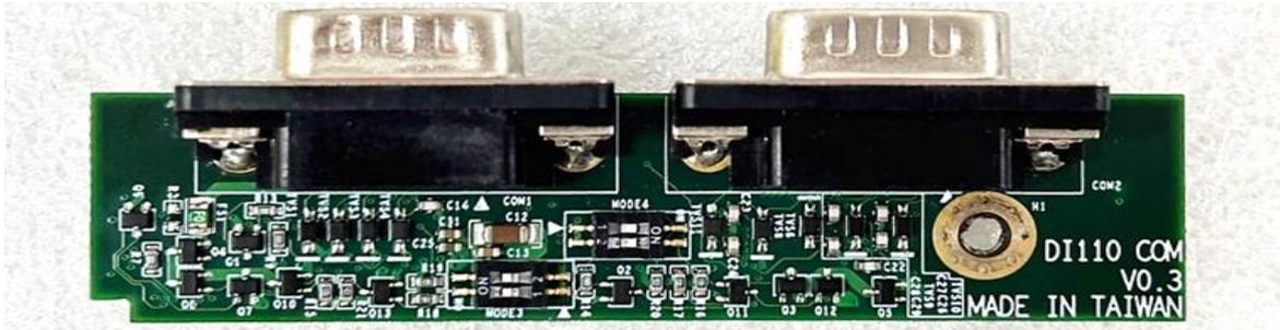
**COM1 and COM2 (on the module) : COM3 and COM4 Connector (Support RS232/RS422/RS485)**
