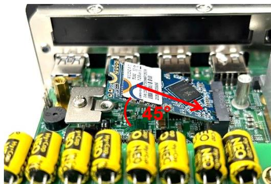
Step 4. Press down the module and fasten the screw to secure the module.
