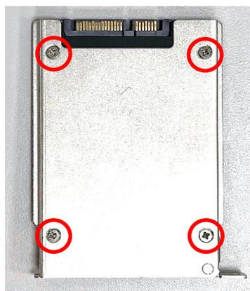
Step 5. Align the HDD bracket with the entrance of HDD bay. And insert the HDD bracket until the connector of HDD contact the SATA connector firmly.
