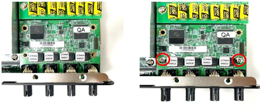
Step 5. Attach the assembled M12 I/O bracket on to the system, and fasten the hex nuts to fix it.
