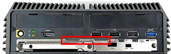
Step 3. Insert the SIM card(s) into the SIM slot(s) with the gold contacts facing up. Please pay attention to the insert orientation as illustrated. (When SIM cards are inserted into both sockets, the network connection will prioritize SIM1.)
