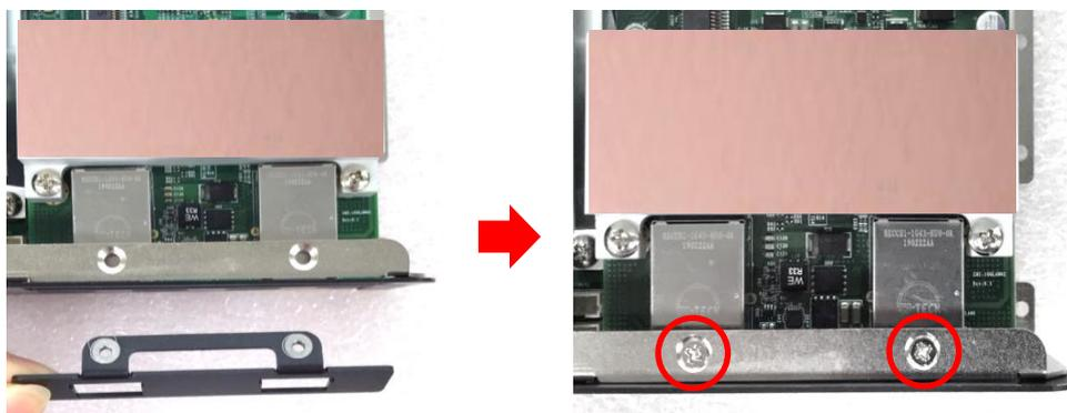
Step 8. Fasten the 4 D-Sub jack screws to fix the module. Then the installation of the module is complete.
