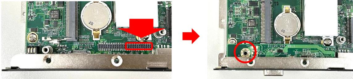
Step 4. Fasten the screw to secure it in place.
