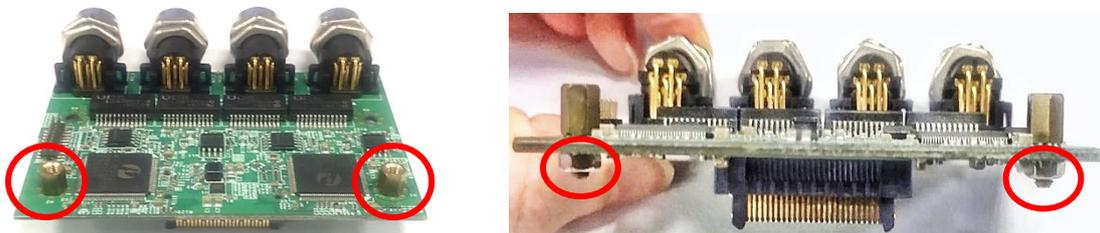
Step 2. Insert the LAN module vertically to the female connector on system's mainboard until it is connected firmly, and fasten the two copper pillars.
