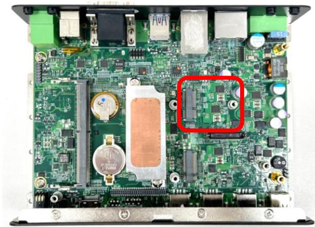
Step 3. Tilt the M.2 Key E card at a 45-degree angle and insert it to the socket until the golden finger connector of the card seated firmly.
