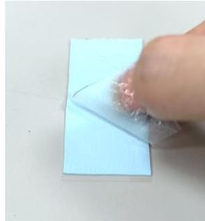
Step 2. Place the thermal pad onto the CPU heatsink, ensuring the peeled side faces downward.
