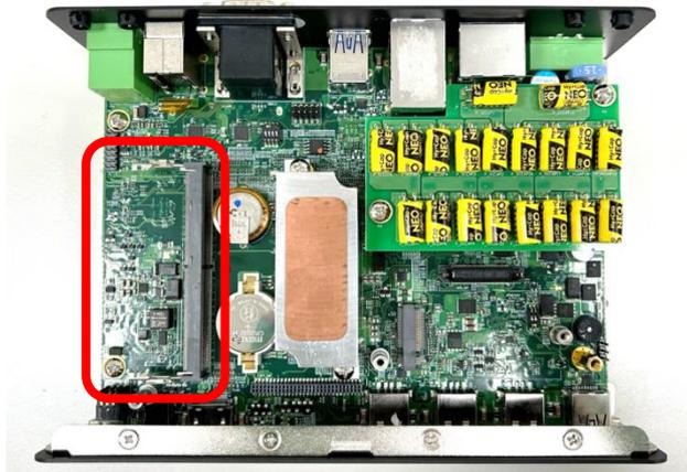
Step 2. Tilt the SO-DIMM module at a 45-degree angle and insert it to SO-DIMM socket until the gold-pated connector of module contacted firmly with the socket.
