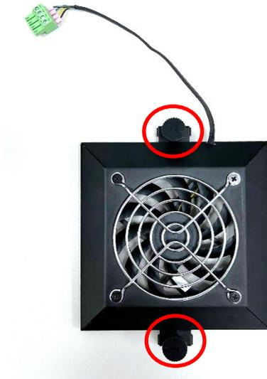
Step 2: Loosen two screws without removing them.
