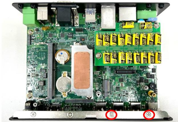
Step 3. Insert the CMI module vertically until it's connected firmly and fasten 2 screws to fix it.
