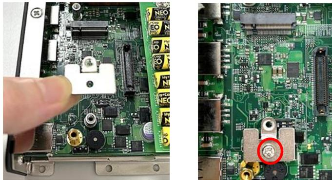
Step 3. Insert the M.2 Key B module at a 45-degree angle and insert it to the slot until the gold-pated connector of module contacted firmly with the slot.
