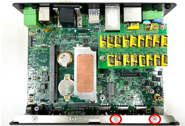
Step 3. Remove the four hex rings from the CMI-M12LAN module.
