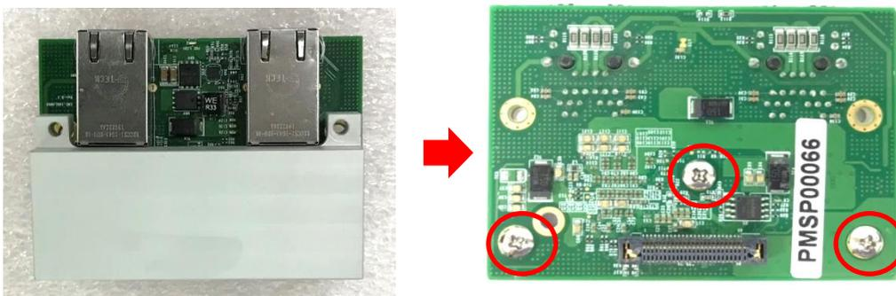
Step 5. Insert the CMI module vertically into the female connector on system's mainboard until it's connected firmly and fasten the 2 screws (M3X12L) to fix it.
