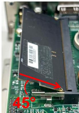
Step 3. Press the modules down until it's fixed firmly by the two locking latches on each side.
