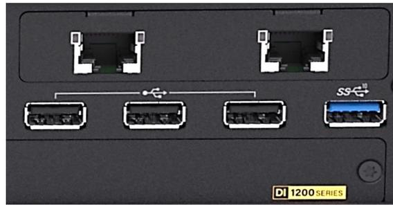
After installing the CMI-10GLAN04-R10 module, users need to enter BIOS > Chipset > [PCH-IO Configuration](#) page, and change the [BTB\_FH1 Mode Selection] setting from default mode [4x1] to mode [1x4] to enable the function of the module.
