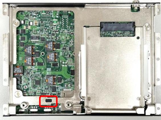
Step 2. Insert the connector of IGN module to the female connector on system motherboard. (Make sure all the pins of IGN module's connector are firmly connected.)
