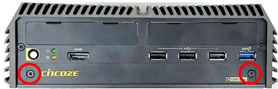
Step 2. Loosen the screw on the HDD bracket.
