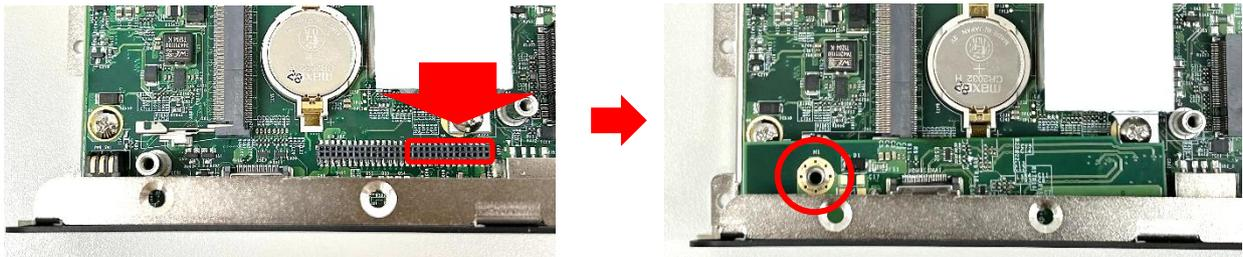
Step 4. Fasten the screw to secure it in place.
