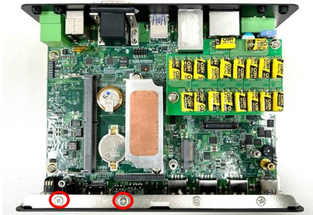
Step 3: Align the pins on the module with the connector on the left side as indicated, and then insert the CMI module vertically until it is securely connected with ensuring that the screw holes are properly aligned.
