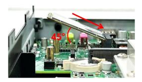
Step 3. Press down the module and fasten the screw to secure the module.
