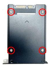
Step 5. Align the HDD bracket with the entrance of HDD bay. And insert the HDD bracket until the connector of HDD contact the SATA connector firmly.
