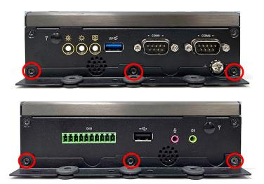
Step 3. Attach the system to the wall by fastening four screws through the mounting holes at each side as illustrated.
