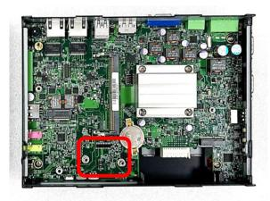
Step 2. Insert CFM-IGN module vertically to the female connector on the system's mainboard, and fasten the 2 screws to fix it.
