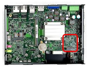
Step 2. Tilt the M.2 Key E card at a 45-degree angle and insert it to the socket until the golden finger connector of the card seated firmly.
