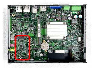
Step 2. Insert the M.2 Key B card at a 45-degree angle and insert it to the slot until the gold-pated connector of module contacted firmly with the slot.
