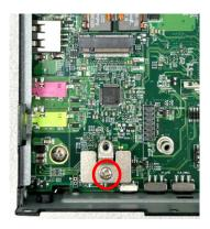
Step 3. Insert the M.2 Key B card at a 45-degree angle and insert it to the slot until the gold-pated connector of module contacted firmly with the slot.
