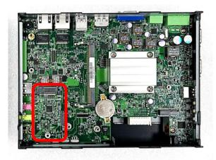
Step 2: Align the M.2 Key B Type 3052 to 3042 Adapter Bracket with the corresponding screw hole. Secure the bracket in place and fasten the screw.
