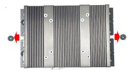
Step 2. Fasten 2 DIN rail mounting clips to mounting brackets on both sides with provided 4 screws (with each screw size of T3x10.5) as illustrated.
