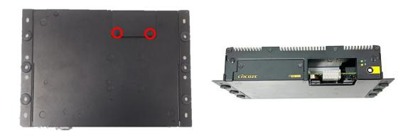
Step 3. Locate the male connector (on the display module) and the female connector (on the system).
