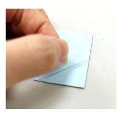
Step 2. Place the thermal pad on the CPU heatsink.
