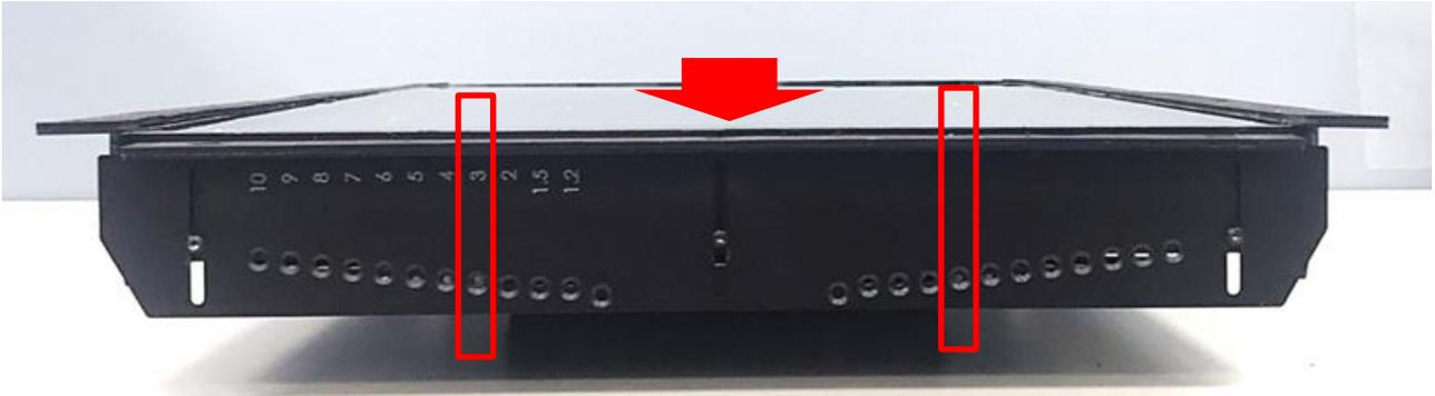
6. Fasten the two screws on the left and right-side mounting brackets.
