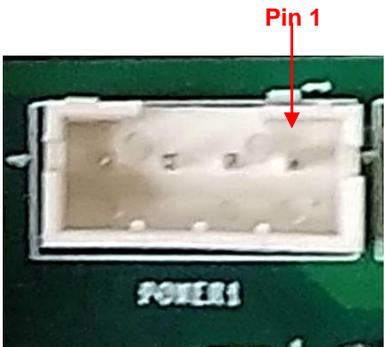
**PWR\_SW1: Remote Power On/Off Switch Connector**
