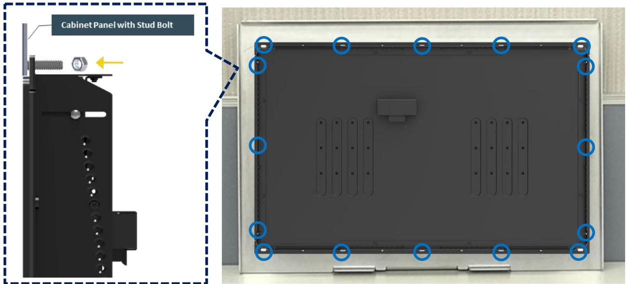
If the cabinet panel is with bosses as the following figures, user can prepare 16 pcs of M4 screws for fixing the module through the **oblong holes** (oblong hole size: 9mmx 4mm, without screw thread).
