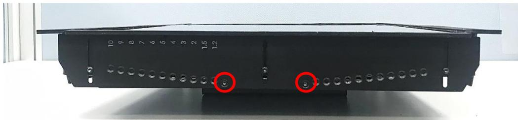
3. Loosen the three screws on the left and right-side mounting brackets.
