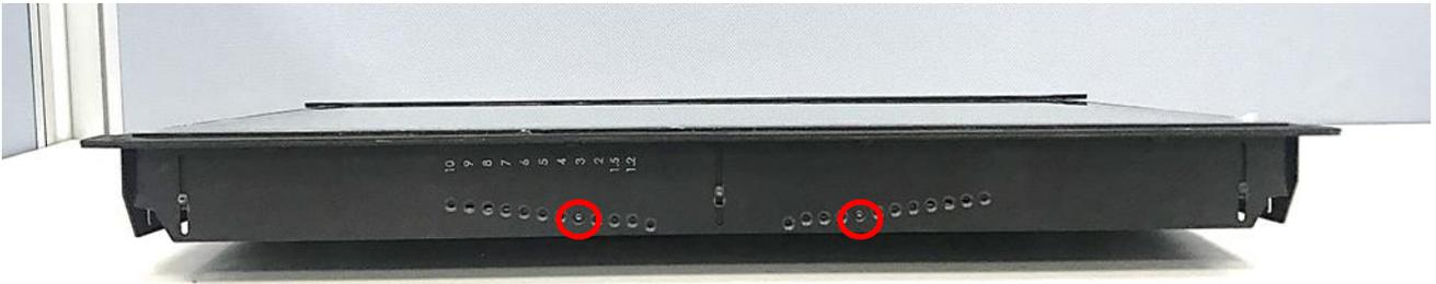
13. Fasten the three screws on the top and bottom-side mounting brackets.
