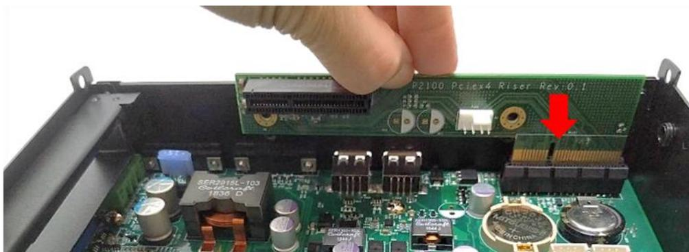
5. Align the notch of golden fingers of PCI(e) card with the expansion slot. Insert the card horizontally, and press the card straight down into the slot until it's seated firmly.
