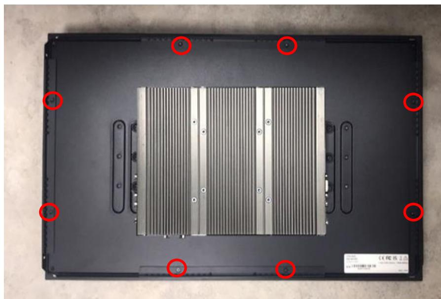
2. Remove the 3 screws on the left and right side of mounting brackets.
