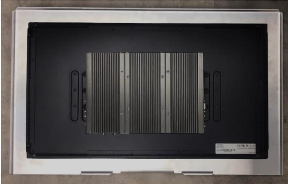
There are two methods for fastening the CO-100/P2102 module onto the cabinet to complete the flat mount. One is to fix the CO-100/P2102 module from the front side of the cabinet, which is illustrated in chapter 3.14.1. The other one is to fix the CO-100/P2102 module from the rear side of the cabinet, which is illustrated in chapter 3.14.2.
