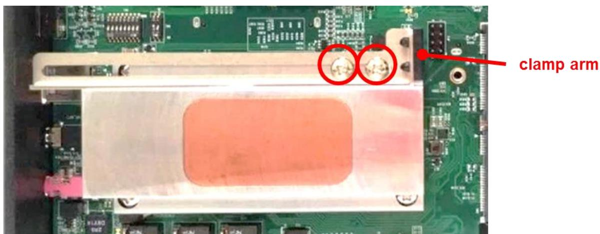
9. Slide the clamp arm of retention module until it contacts the edge of PCI(e) expansion card.
