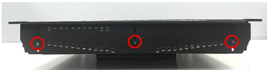
3. Remove the 3 screws on the top and bottom side of mounting brackets.
