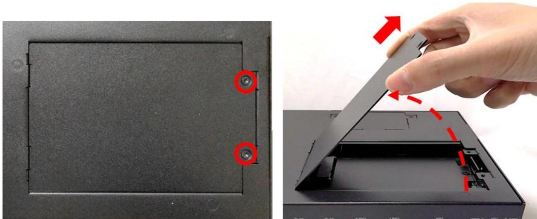
3. Loosen three screws and take the HDD bracket out of HDD compartment.
