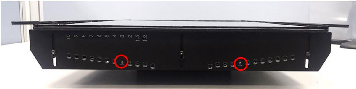
7. Fasten the three screws on the left and right-side mounting brackets.
