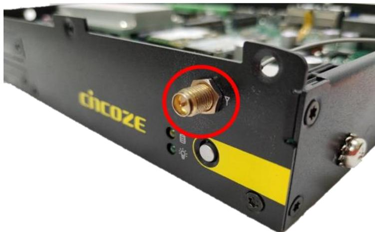
4. Assemble the antenna and antenna jack together.
