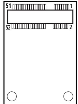
**CN3 : M.2 Key E Socket (Support M.2 PCIE / Intel CNVi )**
