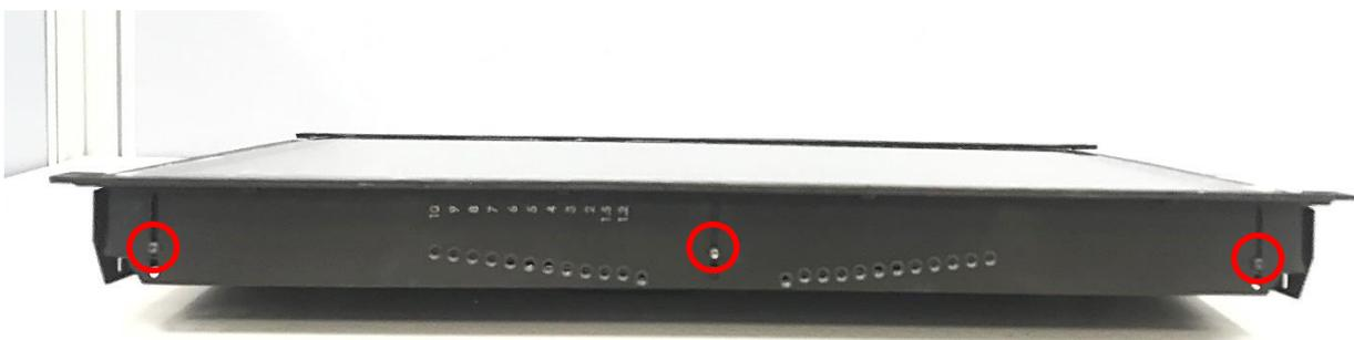
11. According to the thickness = 3mm for the example, push down the top and bottom-side mounting brackets to the place at screw hole = 3mm.
