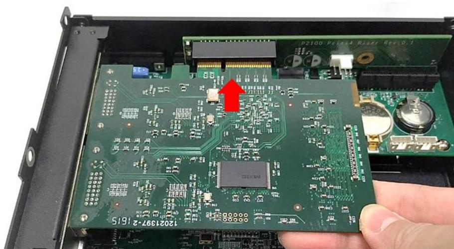
6. Fasten the screw back to secure the PCI(e) expansion card.
