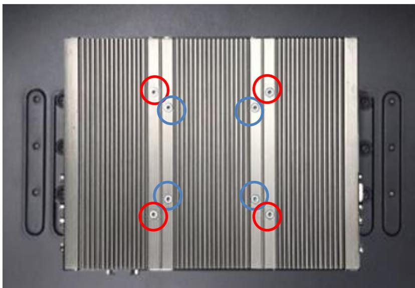
1. Put the VESA stand on, and align with the mounting holes.
