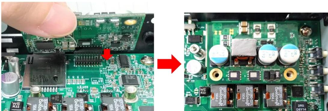
6. Put on the PoE thermal block and fasten two screws to secure the PoE board.
