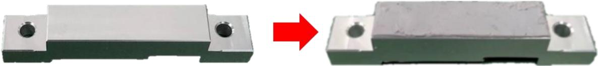
2. Turn over the heatsink and paste the thermal pad at the marked region.
