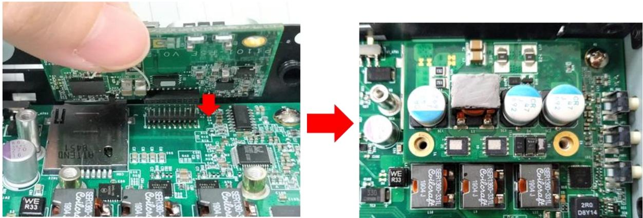
Step 6. Put on the PoE thermal block and fasten two screws to secure the PoE board.
