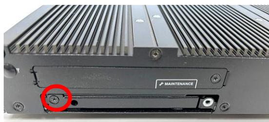
Step 8. Put back HDD bay cover at front panel, and fasten it with the screw.
