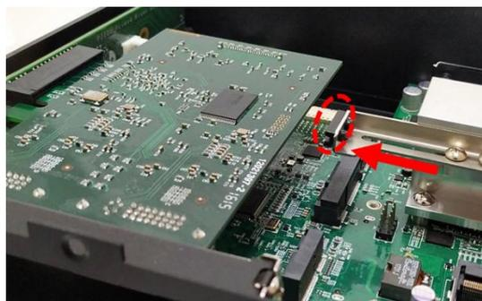
Step 9. Finally, fasten the two screws that were previously loosen halfway to fix the retention module.
