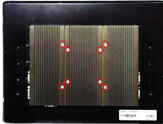
Step 1. The following picture uses a panel PC (P2202+ Display Module) as a demonstration. To attach the panel PC to a VESA stand, please fasten eight screws as indicated to fix it on the stand.
