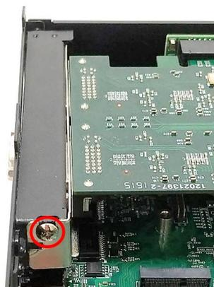
Step 7. Loosen the two screws as indicated to have the clamp arm slidable.
