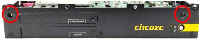
Step 2. Penetrate the antenna jack through the hole. And then put on the washer and fasten the nut with antenna jack.
