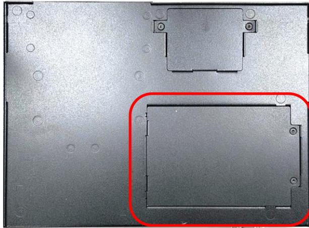
Step 2. Loosen the two screws, lift the cover, and then remove it.
