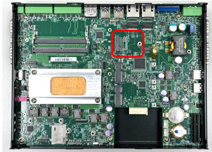
Step 2. Tilt the M.2 E Key card at a 45-degree angle and insert it to the socket until the golden finger connector of the card seated firmly.
