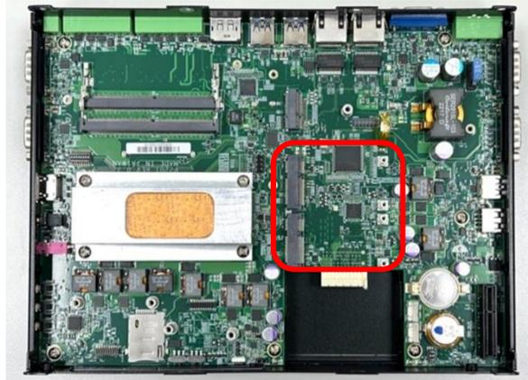
Step 2. Use provided two screws fasten the half size module and adapter bracket together as shown in Fig (a) below.
