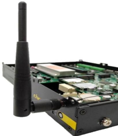
Step 4. Attach the RF connector at another end of the cable onto the card.
