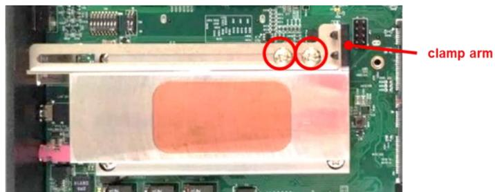
Step 8. Slide the clamp arm of retention module until it contacts the edge of PCI(e) expansion card.
