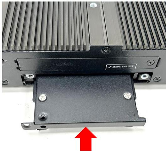
Step 7. Fasten the screw as indicated on the HDD bracket.
