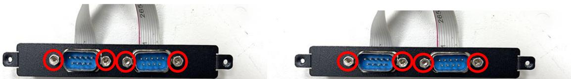
Step 8. Attach the MEC-COM bracket, and fasten the 4 screws to fix it as indicated.
