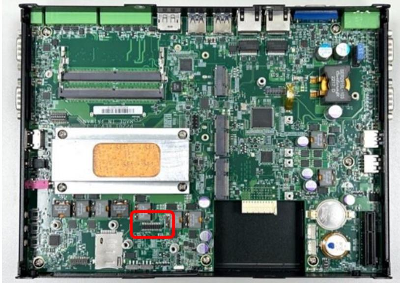
Step 2. Insert the female connector of power ignition board to the male connector on system motherboard.
