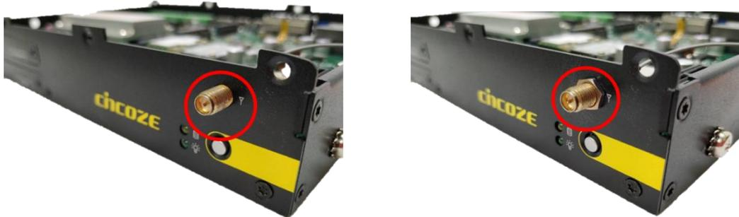
Step 3. Assemble the antenna and antenna jack together.
