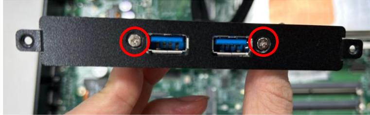
Step 8. Attach the MEC-USB bracket, and fasten the 2 screws to fix it as indicated.
