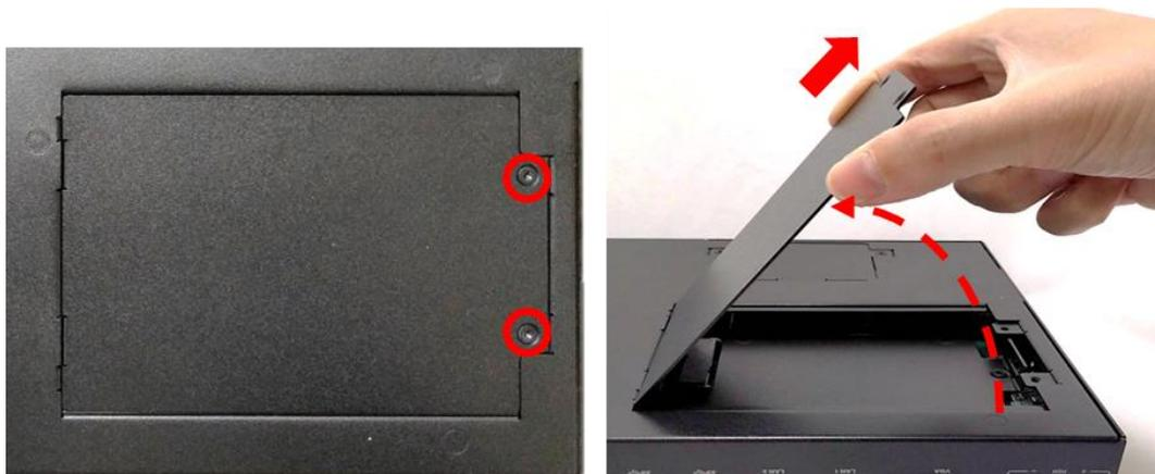
Step 3. Loosen three screws and take the HDD bracket out of HDD compartment.
