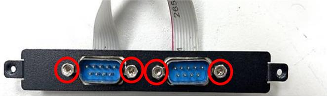
Step 8. Attach the MEC-COM bracket, and fasten the 2 screws to fix it as indicated.
