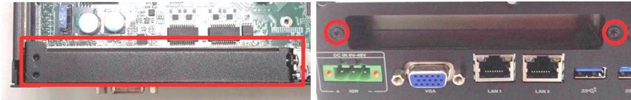
Step 3. Loosen the screw as indicated to remove the PCI bracket.
