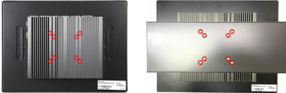
Step 2. Assemble two rack mount brackets by fastening 4 screws (M5x6) at each side.
