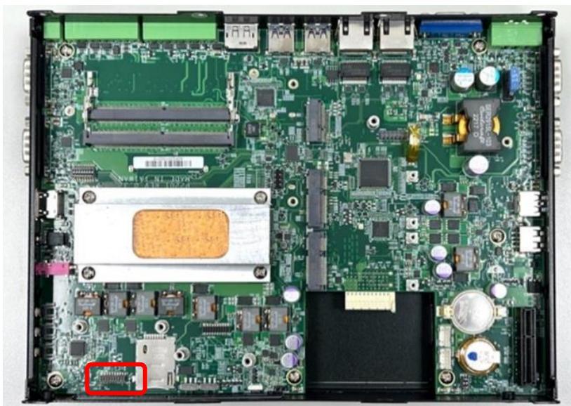
Step 5. Insert the female connector of PoE daughter board to the male connector on system motherboard.
