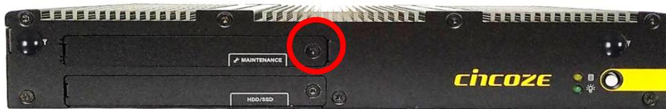
Step 2. Locate the SIM card slot.
