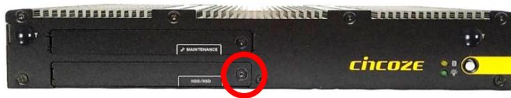
Step 2. Loosen the screw as indicated on the HDD bracket.
