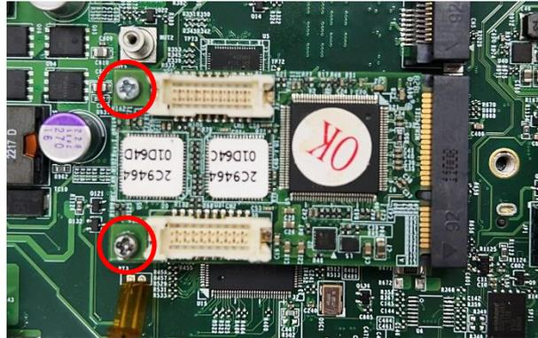
Step 5. Connect the attached wires to the LAN board.
