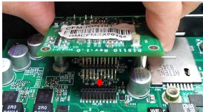
Step 3. Fasten two screws to secure the power ignition board.
