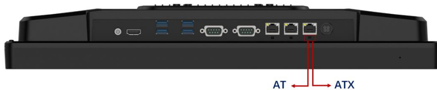
Figure 3-13: AT/ATX Switch Location
