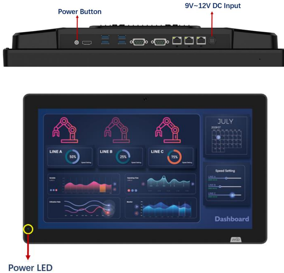
Figure 3-28: Powering On the System
